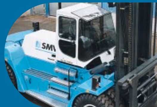
Safety features throughout. Non-slip steps make getting in and out of the cabin easy. The spacing and angle of the steps have been carefully calculated according to official safety studies. The overhead window provides the operator with excellent visibility even when working with the forks in high position. The large, low-cut windshield with all-glass corners provides 180 degrees of unobstructed visibility.
